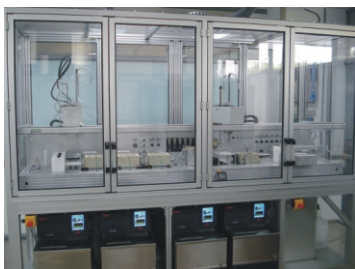
Zinsser High Throughput Polymorph and Salt Screening System at Dr. Reddys Laboratories Ltd and Cipla Limited
