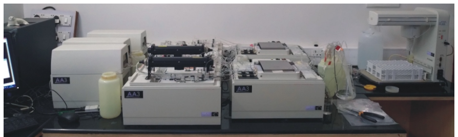
Seal Moduler Auto Analyzer at National Centre for Polar and Ocean Research for Sea Water Analysis
