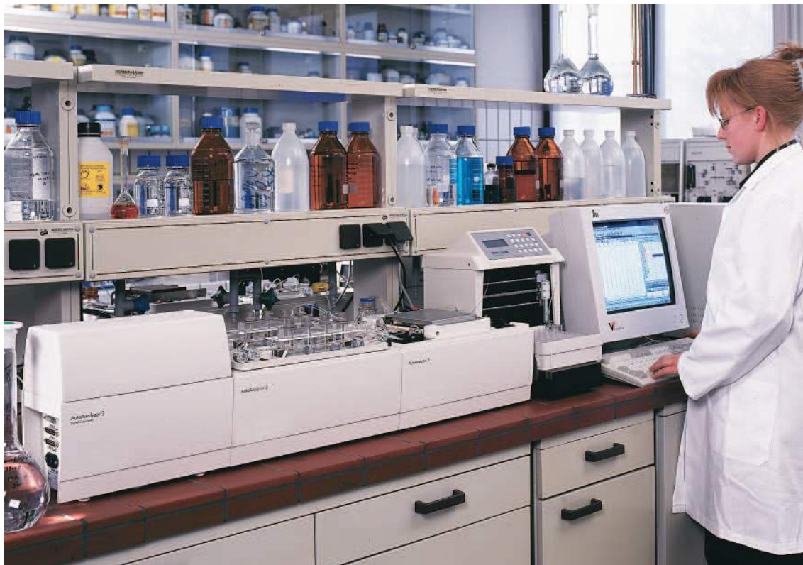
2-channel AutoAnalyzer 3 in a water testing laboratory.
